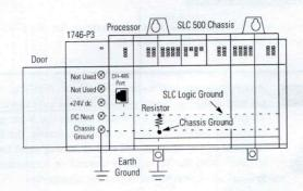
**5. (Optional)** For the 1746-P1, 1746-P2, 1746-P4, 1746-P5, and 1746-P6 power supplies, use PWR OUT +24V dc and PWR OUT COM terminals to power 24V dc sensors and loads. The terminals on the 1746-P1, 1746-P2, 1746-P5, and 1746-P6 power supplies provide an isolated, non-fused 200 mA, 24V dc power supply. The terminals on the 1746-P4 power supply provide an isolated, non-fused 1A, 24V dc power supply. (The 1746-P3 and 1746-P7 power supplies do not provide for an external power source.)
