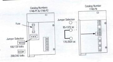
2. Connect the ground screw of the power supply to the nearest ground or ground bus. Use a 1.68 mm (#14 AWG) 75° Copper wire (Category 1 per Industrial Automation Wiring and Grounding Guidelines, publication 1770-4.1) and keep the leads as short as possible. The 1746-P4 is shown
