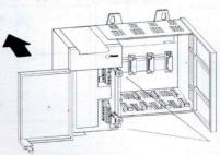
Use these screws to fasten the power supply to the chassis with 1.2 Nm (11 lb-in) torque, max.
