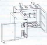
**2.** Slide the power supply in until it is flush with the chassis. Then fasten the power supply to the chassis.
